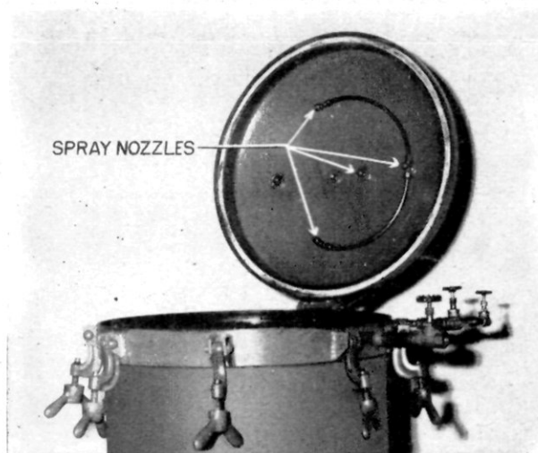
Figure 14.—Location of spray nozzles in retort lid.
