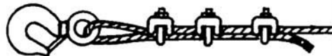
Bad practice – Thimble should be used to increase strength of eye and reduce wear on rope
