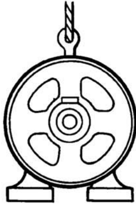
Good practice—vertical lift on eyebolt
